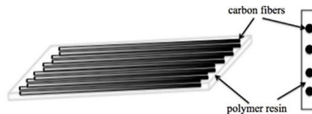
Figure 1. A typical structure of carbon fiber reinforced polymer (CFRP) (Source: ResearchGate.com)
