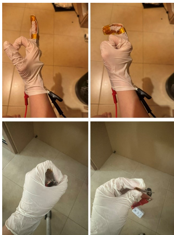
Figure 12: Demonstration of the nanogenerator as motion sensors to detect the motion of finger joints.
