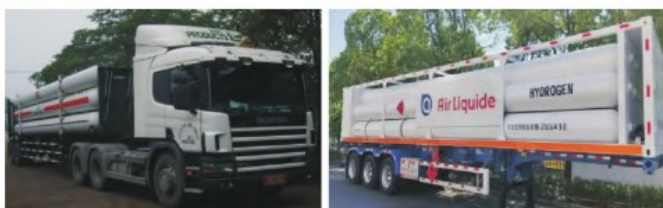
Figure 4: Long tube trailer(left) and tube bundle container(right)
