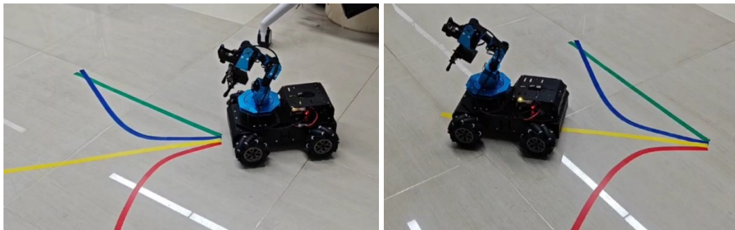
Figure 8: When the voice command is "yellow", the robot performs line-following based on the command.
