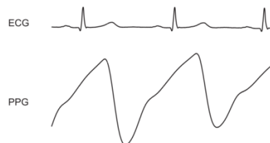
Figure 2: Pulsatile (AC) component of the PPG signal and the corresponding electrocardiogram (ECG)
