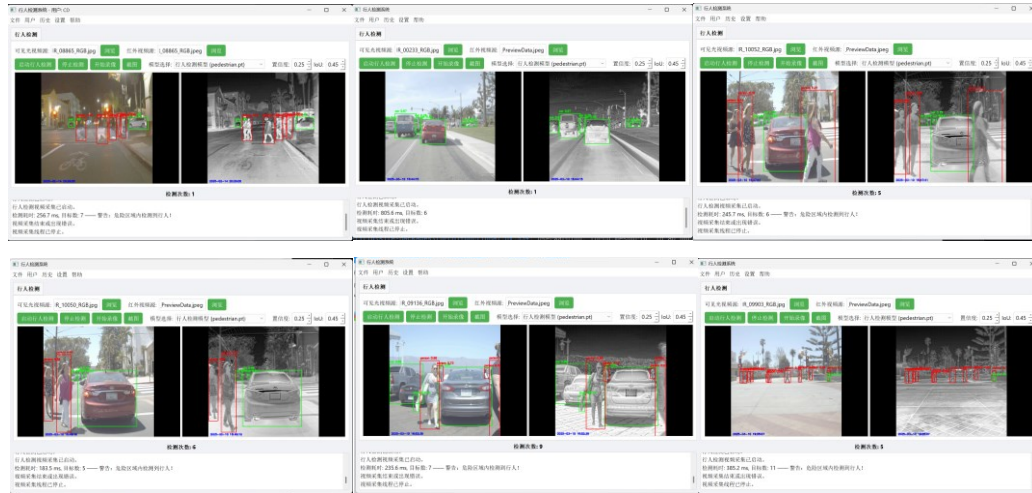
Figure 7: Pedestrian Detection Module Test Results
