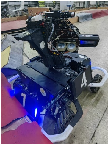
Figure 12: Dual level six friction wheel robot vehicle
