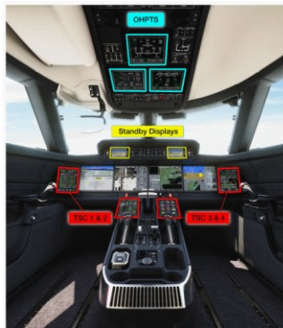
Figure 1: Gulfstream jet uses 10 touch screens
