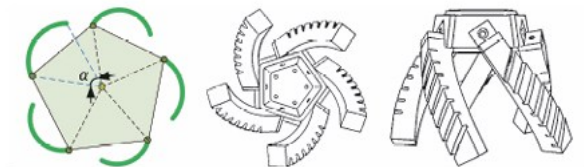
Figure 3: The mechanism of corolla opening and closing movement
