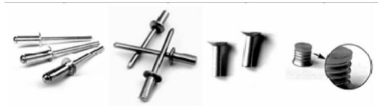
Figure 27. The four types of testing rivets: aluminum-steel BR, aluminum-steel BHR, aluminum alloy COUR, steel SSPR [53]
