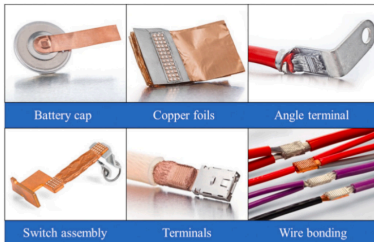
Figure 16. The applications of ultrasonic welding [48]
