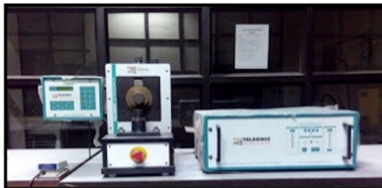
Figure 18. Ultrasonic metal welding device [15]
