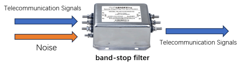
Figure 4. Principle diagram of band-stop filter
