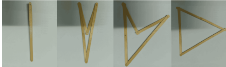
Figure 18. The opening process of a four-bar linkage in one unit
