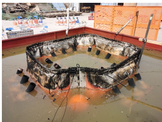
Figure 8. Fire-resistant oil boom after test
