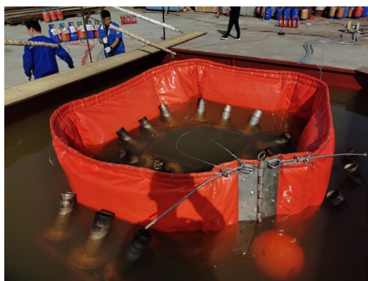
Figure 6. Fire-resistant oil boom placed in the test water tank
