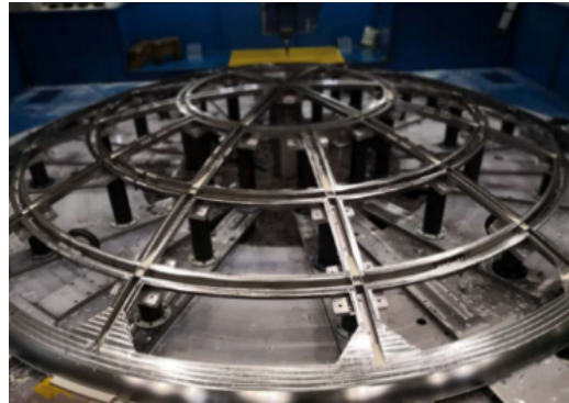
Figure 10. Return capsule heat shield base frame structure
