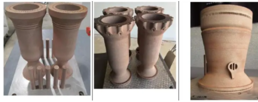
Figure 7. SLM-formed GRCop-84 thrust chamber
