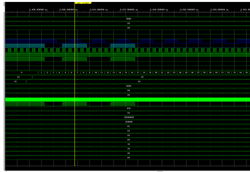
Figure 18. Simulation of IIC master-slave controller on Vivado simulator
