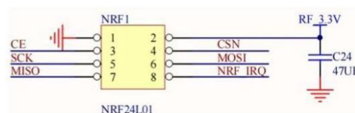
Figure 4. NRF24L01 hardware diagram
