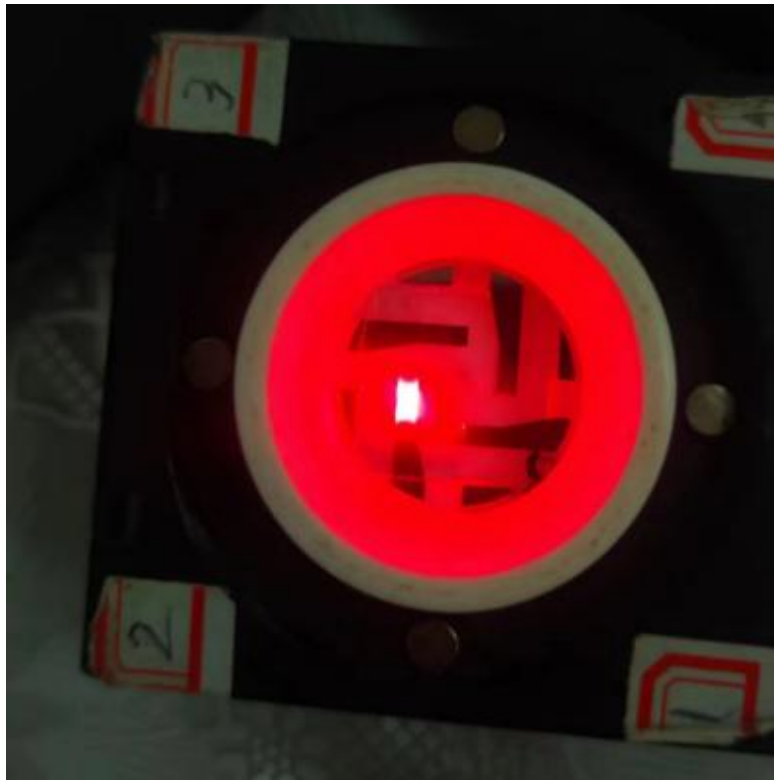
Figure 2. Luminescence diagram of red QLED device
