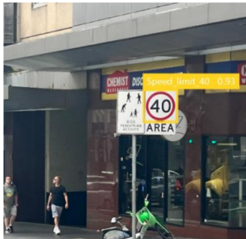
Figure 8. Qualitative detection example of AE-YOLO on a real-world road scene outside the benchmark dataset
