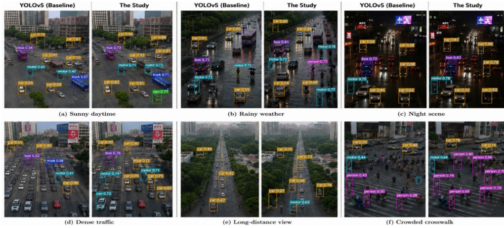
Figure 4. Example of small target detection in different environments (source: VisDrone dataset)
