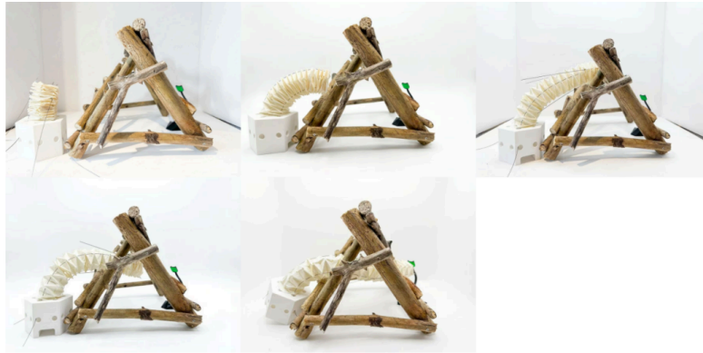
Figure 16. Search-and-rescue test in ruins with origami continuum robot
