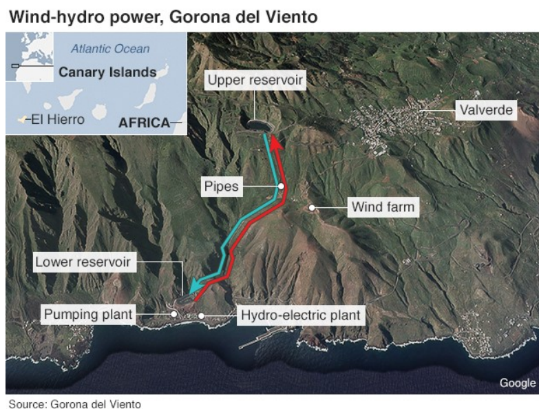
Figure 5. Layout of the Gorona del Viento electric production system. Not shown on the picture is the Llanos Blancos diesel plant located near the coast close to the pumping plant [11]
