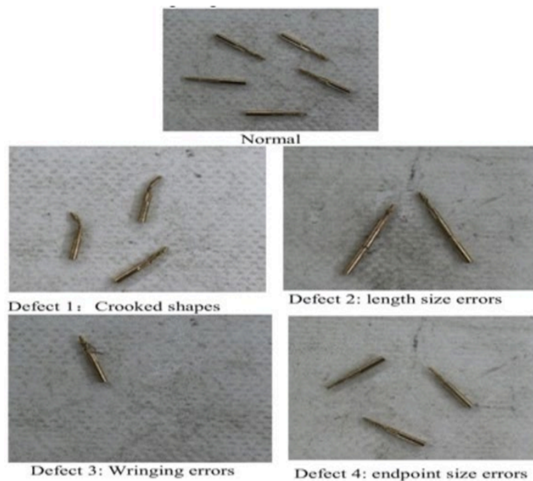
Figure 3. Application of AI in defect detection during SLM 3D printing process
