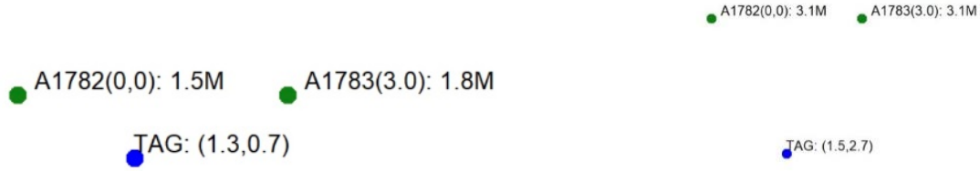
Figure 9. Positioning test using two anchors
