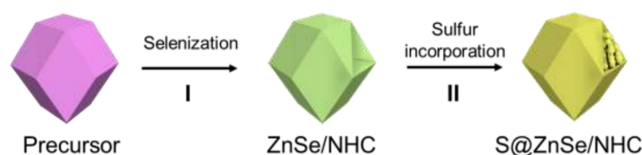
Figure 2. Schematic showing the synthesis procedure of S@ZnSe/NHC composites [5]
