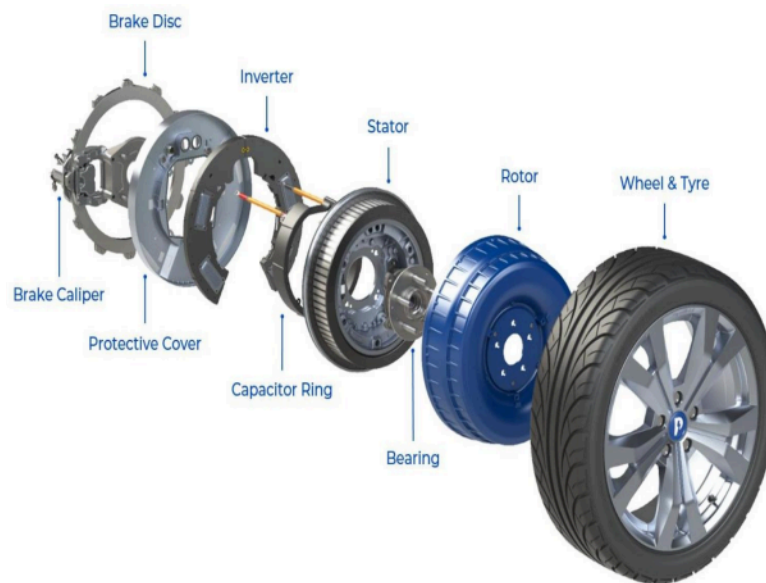
Figure 2. Structure of the Pd18 in-wheel motor
