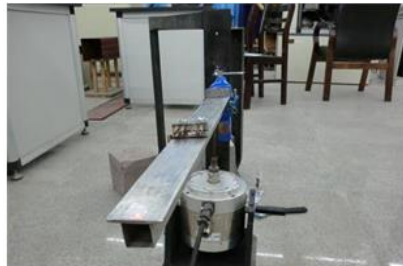
Figure 9. Cantilever beam without SMA material added.
